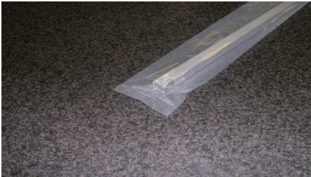
Figure 4. SEALED POLYETHYLENE SLEEVE with FOIL AND POLY SLEEVE TAPED ENDS, READY FOR SHIPMENT
